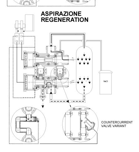
COUNTERCURRENT RINSE VALVE VARIANT COUNTERCURRENT VALVE VARIANT
